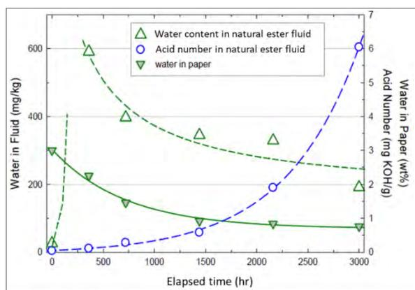
**Figure 3** Results of water content and acid number during the sealed tube ageing test on cellulose paper (pre-aged in mineral oil at 170°C for 400 hours) at 85°C in natural ester
