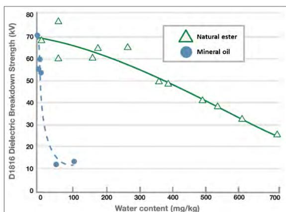
**Figure 4** Dielectric strength of natural ester and mineral oil at different moisture levels
