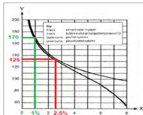
**Figure 5** Temperature threshold for bubble formation on paper insulation surface
