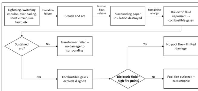
**Figure 1** Sequence of events in transformer failure illustrate the criticality of the dielectric fluid fire point in preventing catastrophic fire breakout
